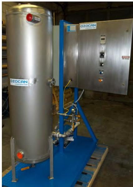
W1 Turn key solution shown includes ozone generator, oxygen generator, mixing vessel, injection venturi, recirculating pump, ozone destructor and skid mounting.
